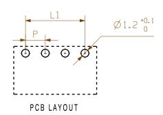
For the mounting of PCBs, it should be noted rated data given in the catalogue relates only to connection elements. The neccessary creepage clearance paths must be observed in connection the respective applicant in accordance to VDE The current-carrying capacity and pitch tolerant be determined according to DIN IEC 326 part
