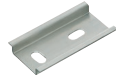
TS 35/7.5 mm according to EN 50022 (s = 1.0 mm)
