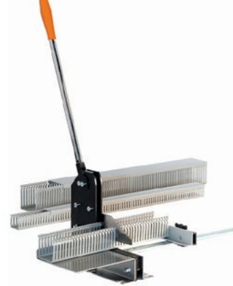
Wire channel cutter for manual operation in cutting wiring channels and covers up to 125 mm wide and a wall thickness of 2.5 mm. Not suitable for plastics reinforced by fillers or halogen-free plastics.
