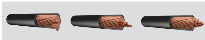
Conductor sheared off Conductor pulled out Squeezed cable
