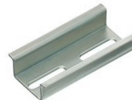
TS 35/15 mm according to EN 50022 (s = 1.5 mm)
