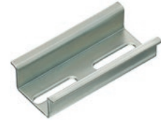
TS 35/15 mm according to EN 50022 (s = 1.5 mm)
