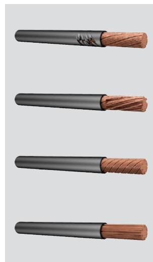
Remains of the conductor insulation are still to be found on the stripped conductor
