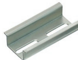
TS 35/15 mm according to EN 50022 (s = 1.5 mm)
