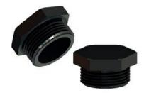
For secure connection of unused screw-in threads or through-hole in enclosures. For Ex e applications with an impact resistance of 7 Joule in accordance with IEC 60079-0.
