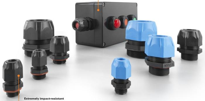
With impact resistance of 7 Joules, the explosion-proof cable glands offer extremely high levels of protection against external influences such as shocks or impacts, in accordance with EN 60079-0:2012 + A11: 2013.
