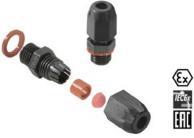
Plastic cable gland for Ex applications with integrated strain relief, especially for Ex e and Ex i applications with silicone seal and 7 Joule impact resistance. Complete with integral membrane seal for clean transportation and storage.
