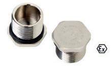
Blanking plug is used for sealing surplus threaded holes to ensure the IP protection degree - especially for Ex-e and Ex-d applications.
