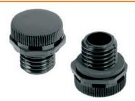
The DAE pressure-compensation element provides good ventilation for the enclosure and prevents moisture build-up. At the same time it maintains the high IP69k protection level. The membrane repels water and oil.
