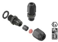
Plastic cable gland for Ex applications with integrated strain relief, especially for Ex e and Ex i applications with chloroprene seal and 7 Joule impact resistance. Complete with integral membrane seal for clean transportation and storage.
