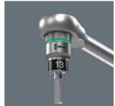
The clamping of the screw is achieved by a twin spring loaded ball retention system. The tubing is effectively protected against mechanical wear and tear by a steel ring. The holding function is especially helpful in confined, hard-to-reach spaces, where there is no room for a second hand to secure the screw.
