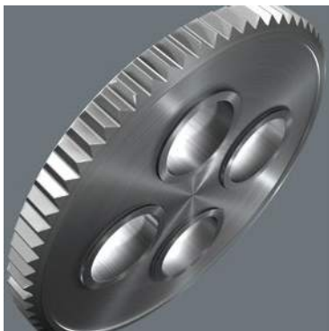
The fine tooth mechanism, with its 60 teeth, allows a small return angle of only 6° – ideal for precision work.
