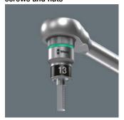
The clamping of the screw is achieved by a twin spring loaded ball retention system. The tubing is protected effectively against mechanical wear and tear by a steel ring. The holding function is especially helpful in confined, hardto-reach spaces, where there is no room for a second hand to secure the screw.
