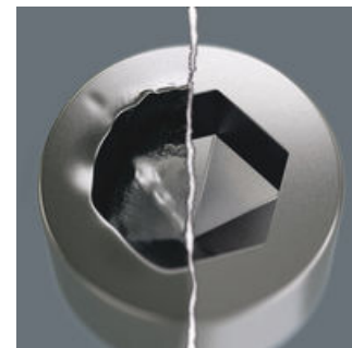
Hexagon screws can endure a problem because the contact surfaces delivering the power from the conventional tool, is transferred to the screw via very small surface areas. The consequence: the screw can become damaged (rounding out). Hex-Plus tools have a greater contact surface that prevents this from happening! At the same time, as much as 20 % more torque can be applied. Good to know: Hex-Plus tools fit into every standard hexagon socket screw!
