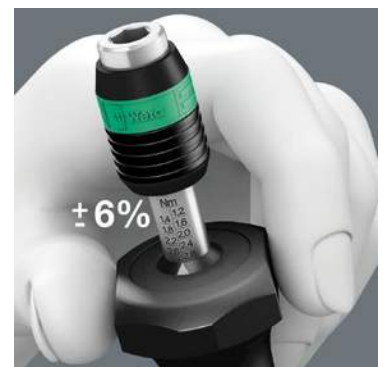
Measurement accuracy is \pm 6\% in accordance with the standard DIN EN ISO 6789. Distinctly audible and noticeable excess-load signal when the pre-set torque is reached.
