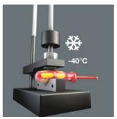
Impact strength tested at  $-40^{\circ}$ C, guaranteeing safety even under extreme conditions.
