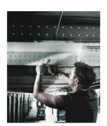
With the Joker, you can now loosen and tighten nuts and bolts, in situations where conventional tools fail. Particularly in confined spaces, where conventional openjawed wrenches cannot be used. The combination of limit stop and small return angle enables eff ective work, even on screw pipe connections.
