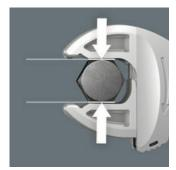
The parallel smooth jaws of the Joker 6004 allow surface pressure and can thus prevent rounding of the bolt or screw head, which can occur during power transmission on corners.
