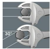
Thanks to the corner-width rectangular prisms, a return angle of only 30° can be realized.
