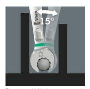
The Joker 6003 ring spanner with its special mouth geometry mouth side pivoted by 7.5° and the double hexagon profile doubles the placement possibilities when repeatedly turning the wrench 180° around the longitudinal axis. Bolts and screw heads can be "accessed" every 15°. The Joker 6003 will automatically find the respective placement point after every turn.
