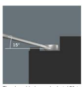
The ring side is cranked at 15° to the tool axis to prevent injury.
