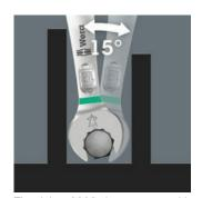
The Joker 6003 ring spanner with its special mouth geometry mouth side pivoted by 7.5° and the double hexagon profile doubles the placement possibilities when repeatedly turning the wrench 180° around the longitudinal axis. Bolts and screw heads can be "accessed" every 15°. The Joker 6003 will automatically find the respective
