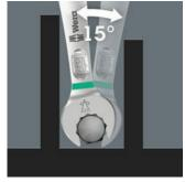
The Joker 6003 ring spanner with its special mouth geometry mouth side pivoted by 7.5° and the double hexagon profile doubles the placement possibilities when repeatedly turning the 180° wrench around the longitudinal axis. Bolts and screw heads can be "accessed" every 15°. The Joker 6003 will automatically find the respective placement point after every turn.
