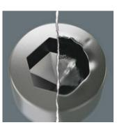
Hexagon screws can endure a problem because the contact surfaces delivering the power from the conventional tool, is transferred to the screw via very small surface areas. The consequence: the screw can become damaged (rounding out). Hex-Plus tools have a greater contact surface that prevents this from happening! At the same time, as much as 20 % more torque can be applied. Good to know: Hex-Plus tools fit into every standard hexagon socket screw!
