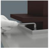
All users will recognise the need to saw or grind down L-keys to make them shorter for particularly confined screwdriving jobs. This has the disadvantage that they no longer have any corrosion protection at the separation point and secondly, they can become "soft" and therefore useless due to an alteration in the hardening during the shortening process.
