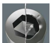
Hexagon screws can endure a problem because the contact surfaces delivering the power from the conventional tool, is transferred to the screw via very small surface areas. The consequence: the screw can become damaged (rounding out). Hex-Plus tools have a greater contact surface that prevents this from happening! At the same time, as much as 20 % more torque can be applied. Good to know: Hex-Plus tools fit into every standard hexagon socket screw!
