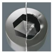
Hexagon screws can endure a problem because the contact surfaces delivering the power from conventional tool, the is transferred to the screw via very small surface areas. The consequence: the screw can become damaged (rounding out). Hex-Plus tools have a greater contact surface that prevents this from happening! At the same time, as much as 20 % more torque can be applied. Good to know: Hex-Plus tools fit into every standard hexagon socket screw!
