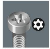
**TORX®** tools with a borehole unauthorised prevent the unfastening of safety screws. The screws contain a pin that protrudes into the drive profile so that "normal" TORX® tools cannot be used. This pin fits into the borehole of TORX® BO tools allowing safety screws to be unfastened.
