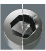
Hexagon screws can endure a problem because the contact surfaces delivering the power from the conventional tool, is transferred to the screw via very small surface areas. The consequence: the screw can become damaged (rounding out). Hex-Plus tools have a greater contact surface that prevents this from happening! At the same time, as much as 20 % more torque can be applied. Good to know: Hex-Plus tools fit into every standard hexagon socket screw!
