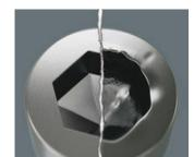
Hexagon screws can endure a problem because the contact surfaces delivering the power from the conventional tool, is transferred to the screw via very small surface areas. The consequence: the screw can become damaged (rounding out). Hex-Plus tools have a greater contact surface that prevents this from happening! At the same time, as much as 20 % more torque can be applied. Good to know: Hex-Plus tools fit into every standard hexagon socket screw!
