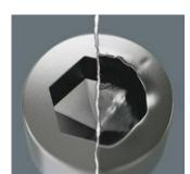
Hexagon screws can endure a problem because the contact surfaces delivering the power from conventional the tool, is transferred to the screw via very small surface areas. The consequence: the screw can become damaged (rounding out). Hex-Plus tools have a greater contact surface that prevents this from happening! At the same time, as much as 20 % more torque can be applied. Good to know: Hex-Plus tools fit into every standard
