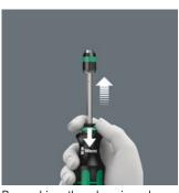
By pushing the clamping sleeve, the telescopic blade can be extended out of the handle and the compact tool becomes a full-sized screwdriver.
