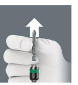
Simply push the sleeve forward to change the bit. The spring mechanism lifts the bit off the magnet and unlocks the tool. The bit can be easily removed. The rapid-out function makes it easy to remove even the smallest bits without extra tools.
