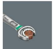
The Joker's clever double-hex geometry delivers a very positive connection with nuts or bolts – it's a perfect fit. And the exchangeable, hardened metal gripping plate in the Joker's mouth literally bites itself into the bolt, with its extremely hard tips. Both features combine to prevent slipping, even at higher torque. 6000 Joker Ratcheting combination wrenches
