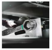
With the Joker, you can now loosen and tighten nuts and bolts, in situations where conventional tools fail. Particularly in confined spaces, where conventional openjawed wrenches cannot be used. The combination of limit stop and small return angle enables eff ective work, even on screw pipe connections.
