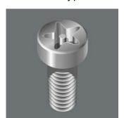
A 5-flank TORX PLUS® profile with a borehole. This drive geometry has only five flanks instead of the usual six and a borehole to protect safety screws against unauthorised unfastening. The screws cannot be turned with conventional, widely available tools.
