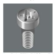
A 5-flank TORX PLUS® profile with a borehole. This drive geometry has only five flanks instead of the usual six and a borehole to protect safety screws against unauthorised unfastening. The screws cannot be turned with conventional, widely available tools.
