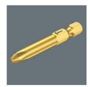
A stands for aviation. A bits are particularly hard bits with a sharp-edged profile which e.g. penetrates screw profiles full of paint (such as on fuselage panels) ensuring a dependable transfer of force between the bit and the screw.
