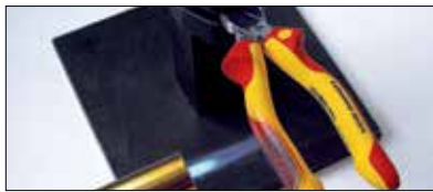
Flame Resistance Test
