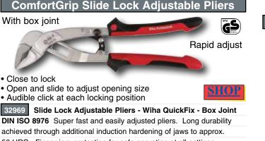
56 HRC. Finger jam protection for safe operation at all settings. Chrome-vanadium tool steel forgings, hardened and tempered. Chrome finish with ergonomic ComfortGrip handles.
