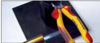
Flame Resistance Test
