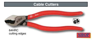
326 Cable Cutters Light, energy-saving & clean cutting with specially ground precision cutting edges. Long life is achieved through additional induction hardening of cutting edge to 64HRC. C70 special tool steel hardened and tempered. Soft vinyl grips. For cutting of copper & aluminum cables without crushing, also suitable for stripping. Not for steel cable, wires and copper conductors with hard coatings.
