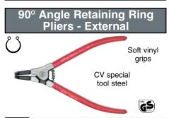
32690° Angled External Retaining RingPliersDIN ISO 5254 Shape B, 90° angledtips. Die forged cylindrical precision formed.For fitting & removing external retaining rings.
