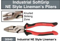
Pliers Long life edge is achieved through additional induction hardening to approx. 64HRC. Special C70 tool steel hardened & tempered. Extra long cutting edge for flat and round cables. Two component SoftGrip handle. Item ÷. No. mm Inch Pkg. wt. 30940 245 9.5 1.18
