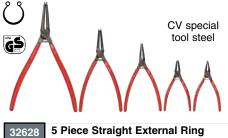
**Pliers Set** Shape A, straight tips. Die forged cylindrical precision formed. CV special tool steel. For fitting & removing external retaining rings. Soft vinyl grips.
