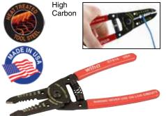
57816Wire Strippers & CuttersSerrated pliers nose for pulling andworking wire. Precision ground strippingstations. Scissors action cutter. Holes in jawfor looping wire. With return spring. Wirestripping stations 10 - 20 / 0.8 - 2.6mm.Item No.mmInchStrips578161526.010-20
