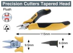
32704 Precision Cutters, Small Tapered Head With Hollow Ground Back, Flush Cutters drop-forged for an ideal material structure. Precise aligned cutting edges are additionally induction hardened at a hardness of Approx. 64°HRC. ESD Safe Dissipative. Item No. mm Inch Copper Head Wdth 32704 115 4.5 1.0 9.5mm
