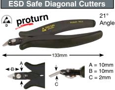
45823 Proturn ESD Safe 21° Precision Cutters/Flush Cut ESD standard IEC 61340-5-1. C70 special tool steel. Glare free, black finish. ESD Safe handle with non-slip grips. Item No. mm Inch AWG Pkg. lbs. 133 5.25 14/1.6mm 1 .14 45823
