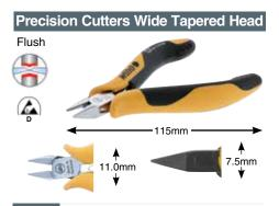
32708 Precision Cutters, Wide Tapered Head, Flush Cutters drop-forged for an ideal material structure. Precise aligned cutting edges are additionally induction hardened at a hardness of Approx. 64°HRC. Two component non-slip soft grip handle, ESD Safe Dissipative. Item No. mm Inch Copper Head Wdth 32708 11.0mm 115 4.5 1.2
