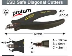
45821 Proturn ESD Safe 45° Precision Cutters/Flush Cut ESD standard IEC 61340-5-1. C70 special tool steel. Glare free, black finish. ESD Safe handle with non-slip grips. Item No. mm Inch AWG Pkg. lbs. 45821 127 5.0 18/1mm 1 .14
