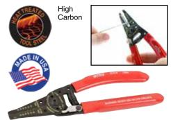
57818Wire Strippers & CuttersPliers nose for working small nuts & pulling<br/>wire. Precision ground stripping stations for<br/>both solid & Stranded wire. Long, curved cutter<br/>requires less force to cut. Holes in the jaw for<br/>looping wire. Return spring & opening stop to<br/>prevent spring from becoming disengaged.<br/>Wire stripping stations 20 - 30 Solid & 22 - 32<br/>Stranded. Screw Cutter 6-32 / 8-32<br/>Item No. mm Inch<br/>57818
