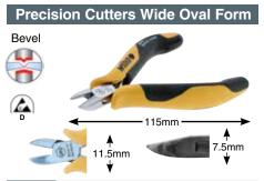
32716Precision Cutters, Wide OvalHead, BevelCutters drop-forged for an idealmaterial structure.Precise aligned cuttingedges are additionally induction hardened at ahardness of Approx.64°HRC.ron-slip soft grip handle, ESD Safe Dissipative.Item No.mmInch CopperHead Wdth327161154.51.411.0mm
