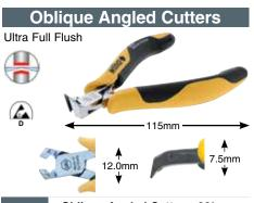
32724Oblique Angled Cutters, 29°,Full Flush Oblique Cutters drop-forged for an<br/>ideal material structure. Precise aligned cutting<br/>edges are additionally induction hardened at a<br/>hardness of Approx. 64°HRC. Two component<br/>non-slip soft grip handle, ESD Safe Dissipative.Item No.mm Inch Copper Head Wdth327241154.51.012.0mm
