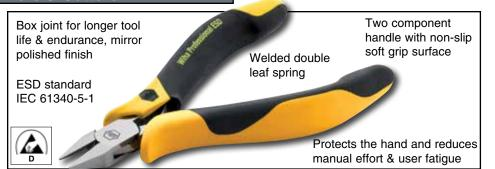
Hardened & annealed high carbon tool steel, induction hardened cutting edges
