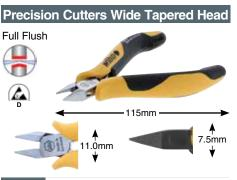
32710 Precision Cutters, Wide Tapered Head, Full Flush Cutters drop-forged for an ideal material structure. Precise aligned cutting edges are additionally induction hardened at a hardness of Approx. 64°HRC. Two component non-slip soft grip handle, ESD Safe Dissipative. Item No. mm Inch Copper Head Wdth 115 4.5 32710 1.0 11.0mm
