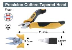
32705 Precision Cutters, Small Tapered Head, Flush Cutters drop-forged for an ideal material structure. Precise aligned cutting edges are additionally induction hardened at a hardness of Approx. 64°HRC. Two component non-slip soft grip handle, ESD Safe Dissipative. Item No. mm Inch Copper Head Wdth 32705 115 4.5 1.0 9.5mm
