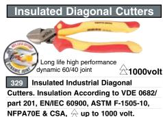
Individually Tested. DIN ISO 5749 Item Cutting Capacity No. Inch Copper AWG lbs. Pkg. mm 32933 160 6.3 #6 .64 1 32929 200 8.0 .80 1 #6
