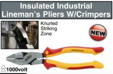
32948 Insulated Industrial Lineman's Pliers With Crimpers. Insulation According to EN/IEC 60900, ASTM F-1505, NFPA70E and CSA,  $\leftrightarrow$  up to 1000 Volt. Individually Tested. Long life edge is achieved through additional induction hardening to approx. 64HRC. Special C70 tool steel hardened & tempered. Extra long cutting edge for flat and round cables.
