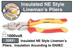
60900, ASTM F-1505, NFPA70E and CSA,  $\Leftrightarrow$  up to 1000 Volt. Individually Tested. Long life edge is achieved through additional induction hardening to approx. 64HRC. Special C70 tool steel hardened & tempered. Extra long cutting edge for flat and round cables. Two component soft grip ergonomic handles.
