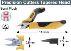
32702 Precision Cutters, Small Tapered Head With Hollow Ground Back, Semi Flush Cutters drop-forged for an ideal material structure. Precise aligned cutting edges are additionally induction hardened at a hardness of Approx. 64°HRC. Two component non-slip soft grip handle, ESD Safe Dissipative. Item No. mm Inch Copper Head Wdth 32702 115 4.5 1.0 9.5mm
