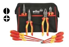
32892 10 Piece Pliers & Screwdriver Set. Insulation According to VDE 0682/part 201, EN/IEC 60900, ASTM F-1505, NFPA70E & CSA, A up to 1000 volt. Individually Tested. In canvas tool bag Item#32892 Set Includes: **↓** lbs. 6.64 8.0" Bent Nose 8.0" Combination Pliers 6.3" Long Nose 6.3" Side Cutters Insulated Slotted 3.0, 4.5, 6.5mm Insulated Phillips #0, 1, 2
