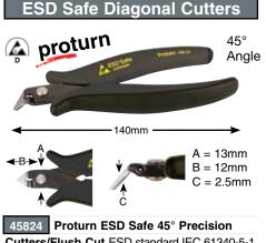
Cutters/Flush Cut ESD standard IEC 61340-5-1. C70 special tool steel. Glare free, black finish. ESD Safe handle with non-slip grips. Item No. mm Inch AWG Pkg. lbs. 45824 140 5.5 14/1.6mm 1 .16
