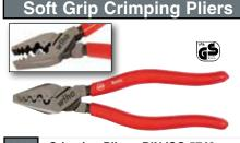
326 Crimping Pliers DIN ISO 5743 Semi-circular profiles for secure connection between end sleeve and conductor. Long life is achieved through additional induction hardening to 64HRC. C70 special tool steel hardened & tempered. Soft vinyl grips.
