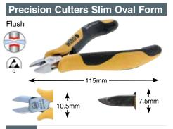
32712Precision Cutters, Slim Oval Head,Flush Cutters drop-forged for an ideal materialstructure. Precise aligned cutting edges areadditionally induction hardened at a hardnessof Approx. 64°HRC. Two component non-slipsoft grip handle, ESD Safe Dissipative.Item No.Item No.mm Inch Copper Head Wdth32712115 4.51.010.5mm
