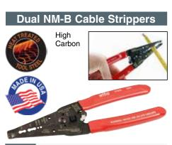
**57820** Wire Strippers Dual NM-B Cable Dual cable stripper features serrated pliers nose, wire looping holes, spring return and lock. Staggered cutting blade produces clean, sure cut with 30-50% less effort. Strippers Size 12-2 / 14-2 NM-B. 12-14 AWG. Screw Cutter 6-32 / 8-32.
