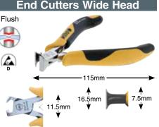
32734End Cutters, Wide Head, FlushEnd Cutters drop-forged for an ideal materialstructure. Precise aligned cutting edges areadditionally induction hardened at a hardnessof Approx. 64°HRC. ESD Safe Dissipative.Item No.mmInch CopperHead Wdth327341154.51.411.0mm
