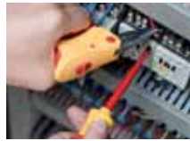
Needle nose pliers Inomic® VDE with cutting edge and stripping points Page 257
