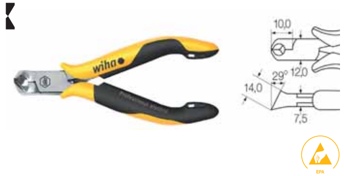
wide head, approx. 29° with small bevelled edge Z 46 1 04
