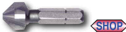
786 HSS 1/4" Drive 90° Countersinks High quality HSS steel, ground with radial relief. 1/4" Hex shank according to DIN 3126 C 6.3.
