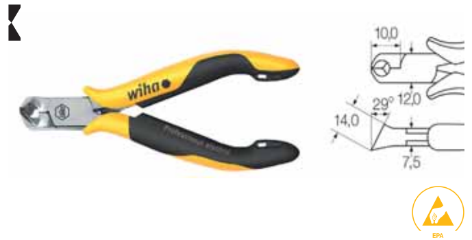
wide head, approx. 29° with small bevelled edge Z 46 1 04
