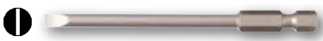
760 Slotted Power Blades S2 modified tool steel. Hardened & tempered to HRC 60. Blades fit CentroFix power blade handle. OAL 90mm/3.5".
