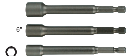
70492 3 pc. Hex Inch Nut Setter Set Permanent industrial magnet. 152mm OAL
