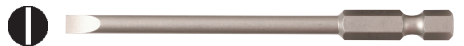
760 Slotted Power Blades S2 modified tool steel. Hardened & tempered to HRC 60. Blades fit CentroFix power blade handle. OAL 90mm/3.5".
