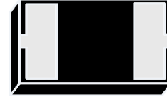
DFN1006-2L (Bottom View)
