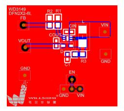
Figure 4, WD3149 PCB Layout with Snubber
