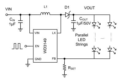
Figure 7, Li-Ion Driver for Parallel White LED Strings
