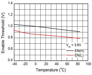
**Enable Threshold vs. Temperature**
