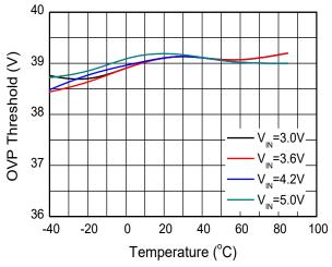
**OVP Threshold vs. Temperature**
