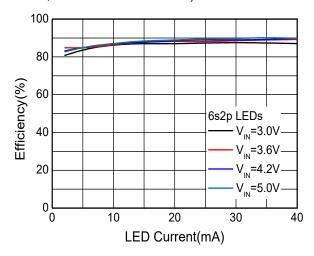
Efficiency vs. LED Current
