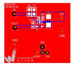
Figure 3, WD3149 PCB Layout Demo
