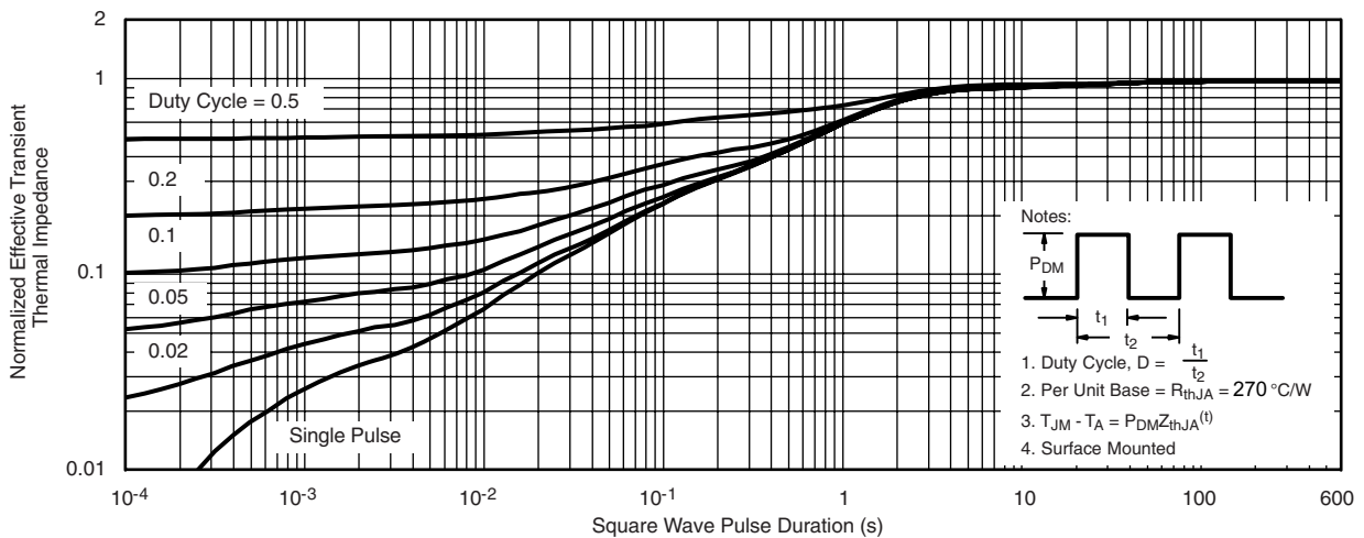
Transient thermal response (Junction-to-Ambient)
