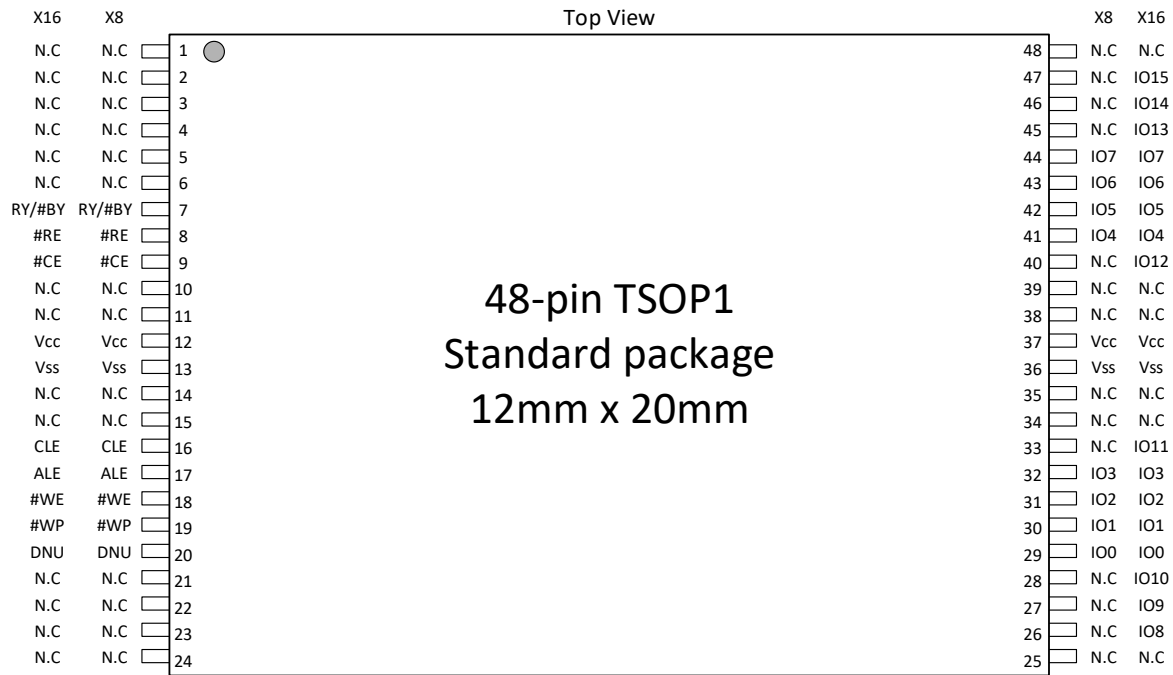
Figure 3-1 Pin Assignment 48-pin TSOP1 (Package code S)
