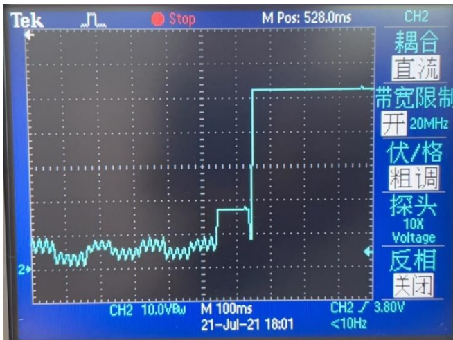
Noise (VIN = 48V, IO = 1.2A, 5 ~ 20MHz bandwidth)
