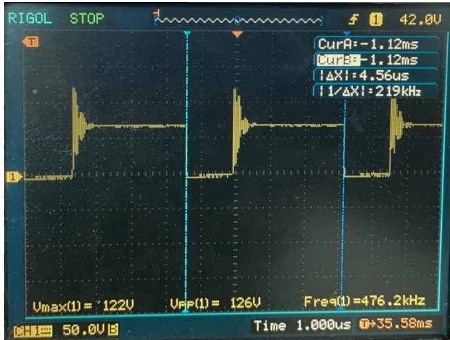
Transformer Switch Waveform
