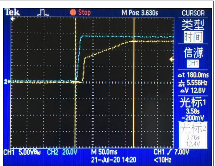
Output response & load (12V / 0.02A)
